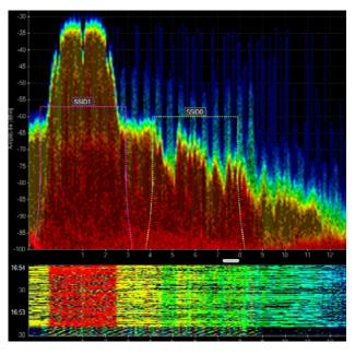
Chanalyzer brings simplicity and power to wireless troubleshooting. It combines Wi-Spy's ability to read raw RF data with your computer's built-in WiFi card to show you how environmental WiFi saturation and non-WiFi transmitters affect your network. Chanalyzer is capable of displaying activity in the 2.4 GHz band, 5 GHz band, or both simultaneously if using Wi-Spy DBx or a Cisco access Point.
