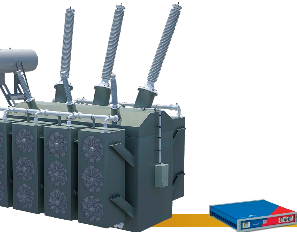
DIRANA determines the moisture content of oil-paper insulated power and instrument transformers and also assesses the condition of bushings by using dielectric response analysis.
